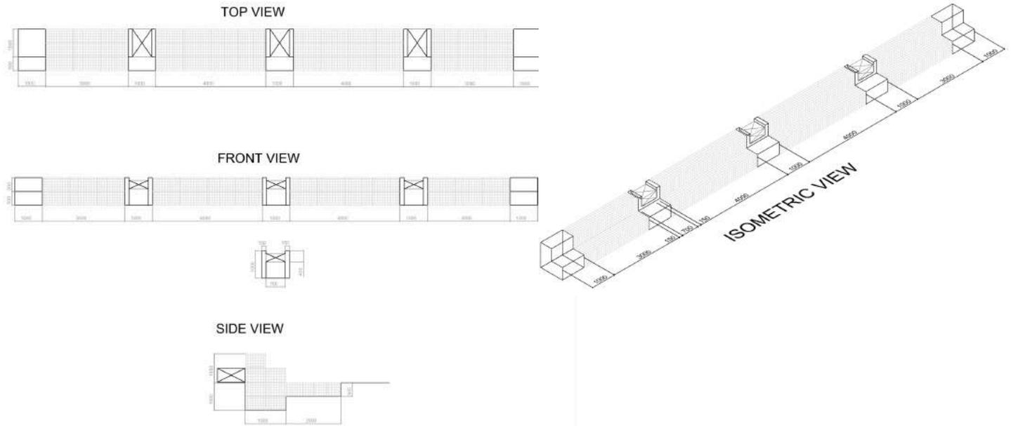
Figure 5. CAD Generated Plan of the Check Dam (Scaled)
